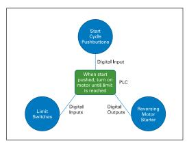
Figure 2. A Simple Motor Control Example of the Basic Control System
