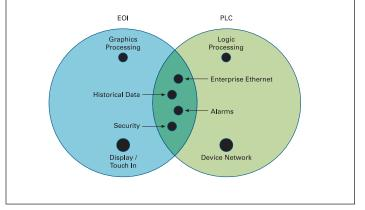
Figure 8. Emerging Overlap of EOI and PLC Features.
