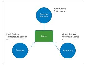
Figure 1. The Basic Components of a Control System
