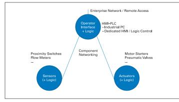
Figure 6. Emerging Lean Automation Architecture
