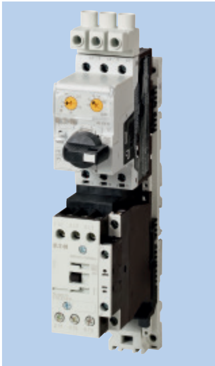
Figure 7: Self-Protected Combination Starter, UL 508 Type E for motor-protective circuit-breakers PKE up to 32 A a contactor is always required.
