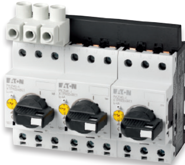
Figure 8: A group of PKZM0 manual motor controllers is linked via a common link bus connector. The controllers are fed by a common BK25/3-PKZ0-E terminal block. The incoming terminal's large electrical clearances at the point of supply enable the entire assembly to meet self-protected "Construction Type E" requirements. The circuit breakers' thumb grips must be lockable.
