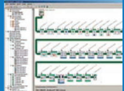
The SWD-Assist software supports users in the planning, engineering, and commissioning of a SmartWire-DT network.
