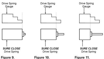
The breaker is set at the factory for an application of one MOC switch. This means that for cell applications with either no MOC switches or one MOC switch, no field adjustments to the *SURE CLOSE* mechanism have to be made. From our records, this about 90% of the applications, as shown in Table 1.
