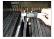
Fig. 1: Measuring the pressing edge
