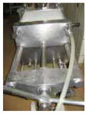
Fig. 7: Central spindle fully screwed in
