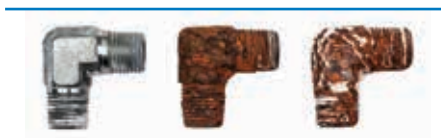
Corrosion of current carbon steel adapters after 650 hours of exposure to salt spray testing.
