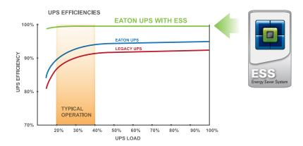
Even at light loads, where you would expect efficiency to be much lower, this UPS maintains a consistently high efficiency profile.
