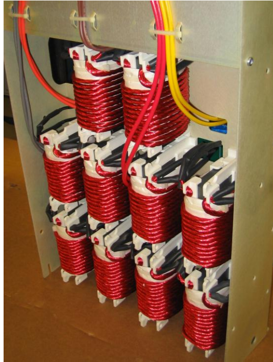
Picture 2: Inductors for half of a complete powertrain of the transformerless topology.
