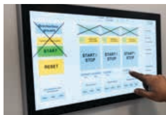
Visualization at the control panel is based on a modern touch panel with capacitive multi-touch technology.
