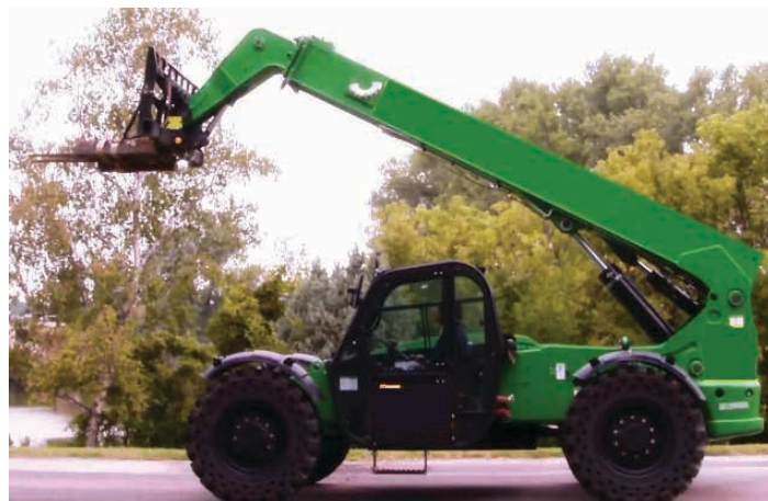
Figure 3: A telehandler was used to test valves under typical operating conditions.
