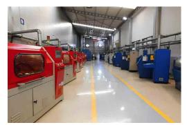
Static impulse tests, full and half omega shape tests, with rotating manifold (special requirement for some customers) can be performed. Standard reporting, according to ISO make the results easy to follow.
