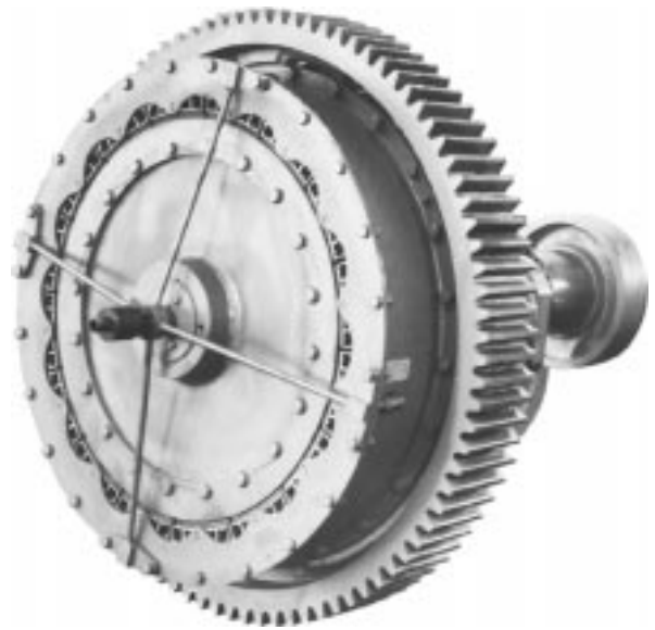
46VC1200 clutch in an air bridge mounting on crankshaft bullgear - 600 ton press, 6 inch stroke.
