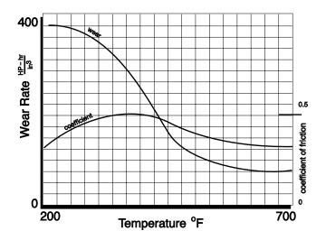
often exceed 1000°F (540°C). Prolonged exposure causes the friction material binder to break down at the surface, resulting in loss of coefficient of friction (lining fade). The clutch or brake can no longer develop its rated torque. Lining wear increases rapidly. The graph illustrates characteristic temperature effects on lining coefficient and wear.
